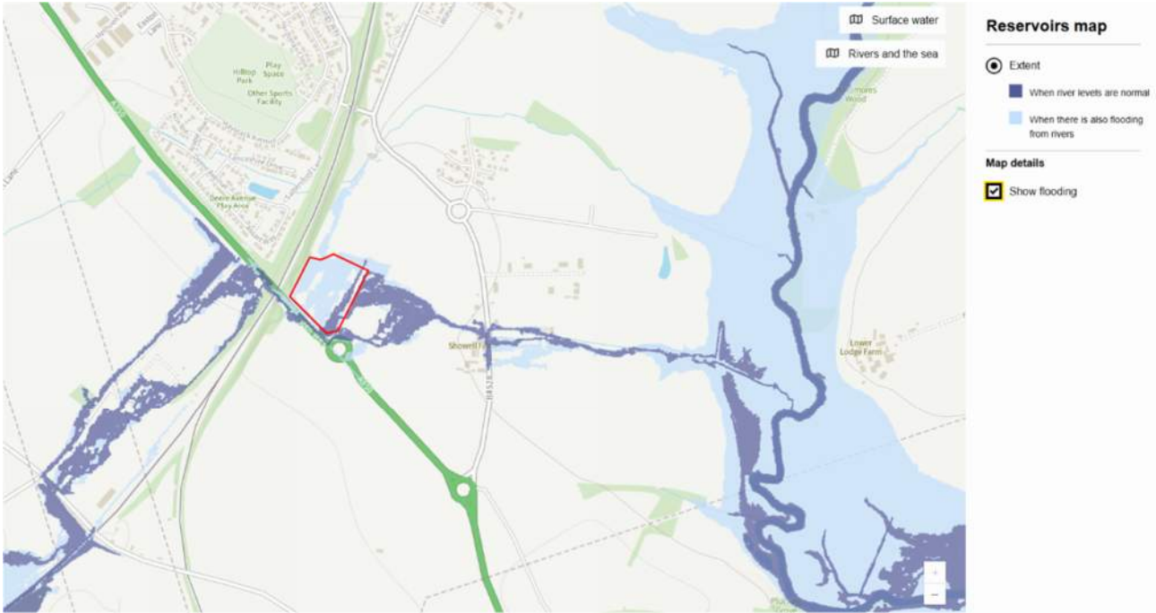
Figure 7: Reservoir Flooding Extent
