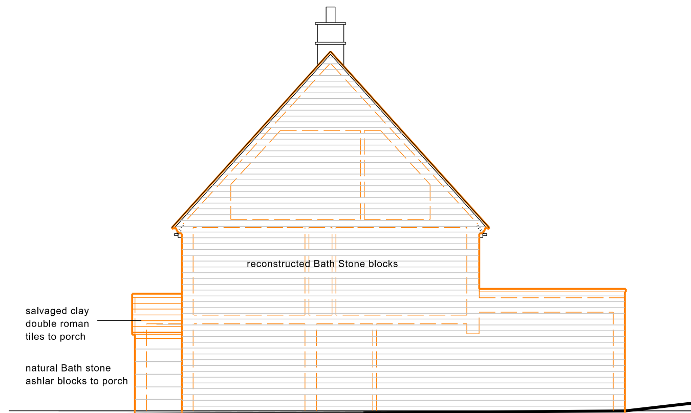
SIDE NORTH ELEVATION
