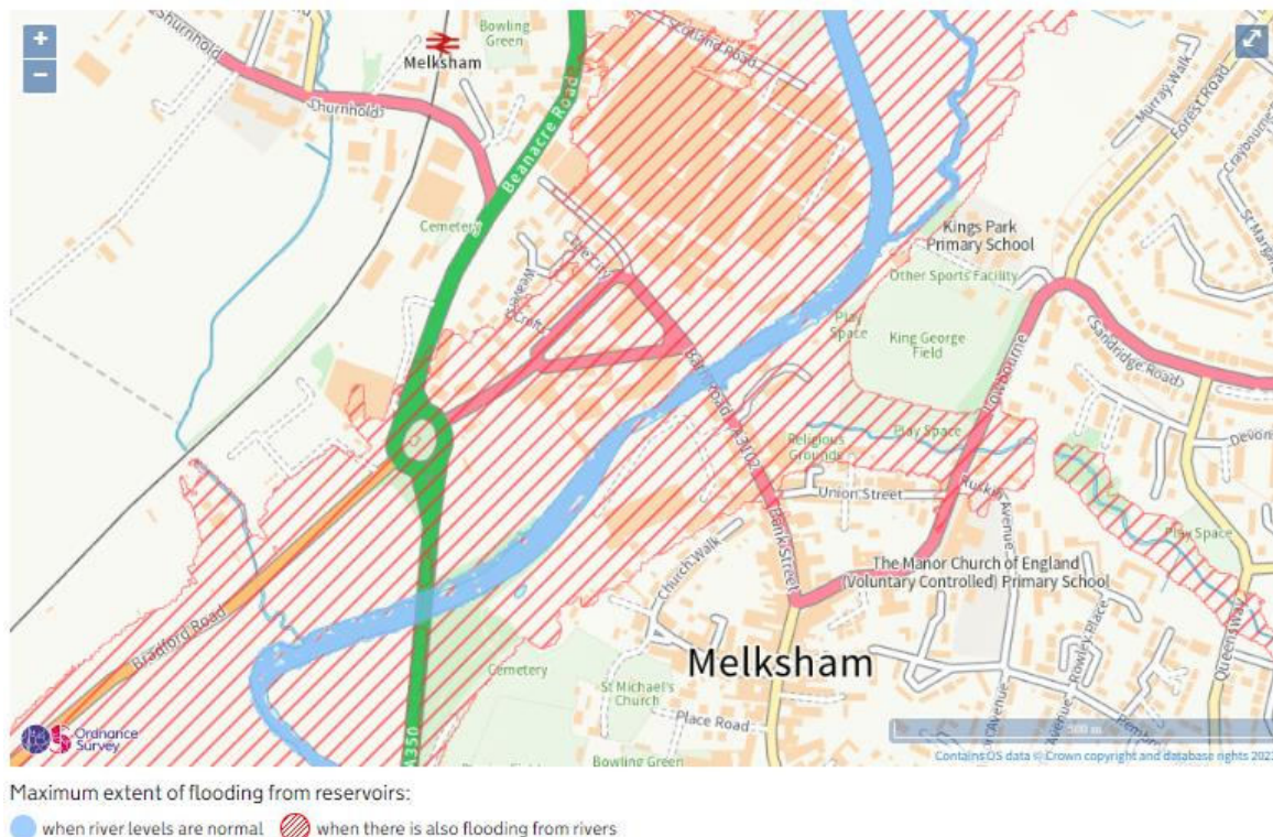
Figure 4: Extent of Flooding from Reservoirs
