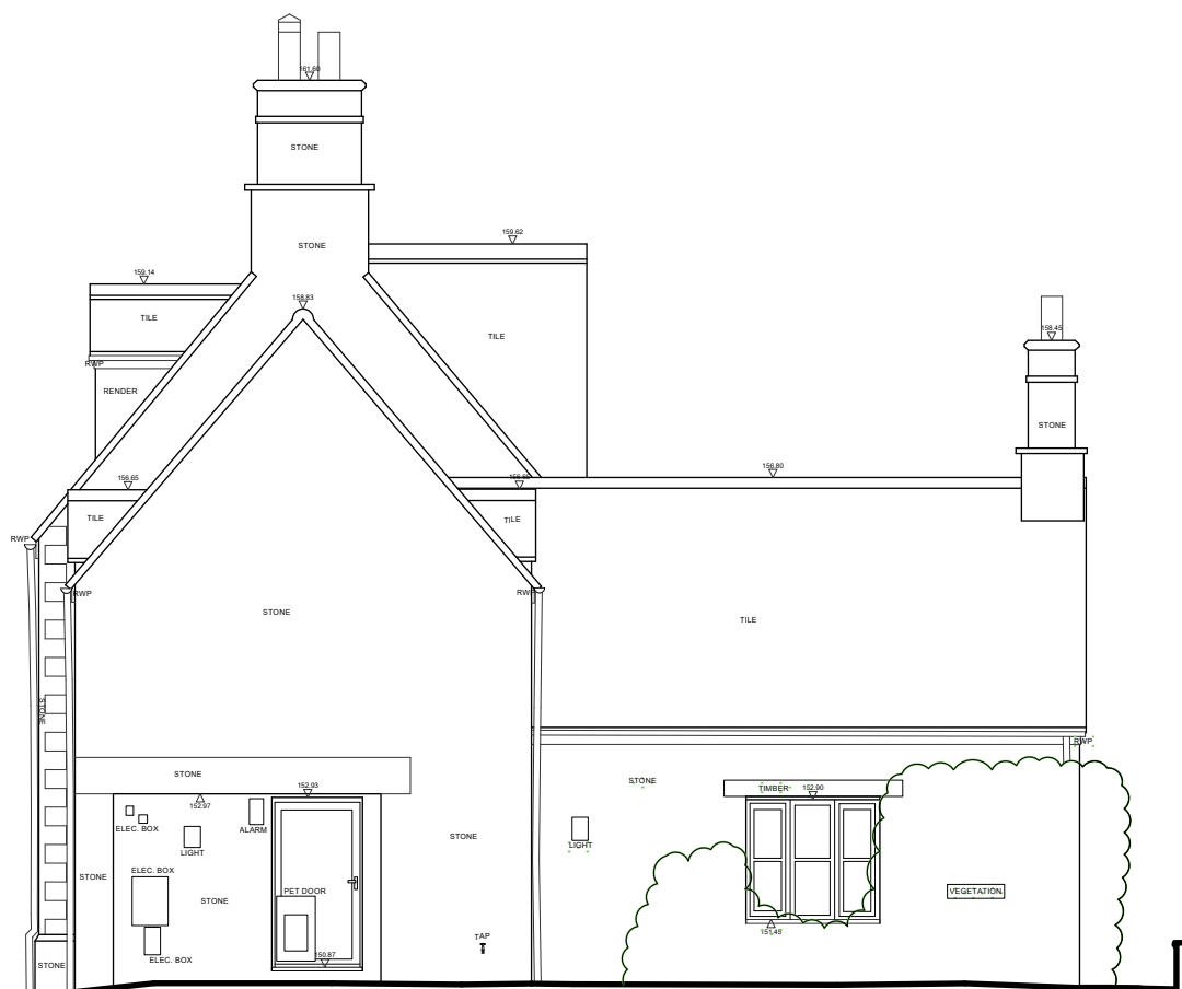
North West Elevation 1:100
