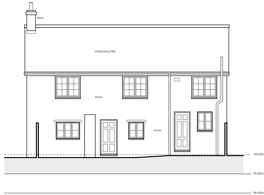
Existing North-East Elevation 1:100
