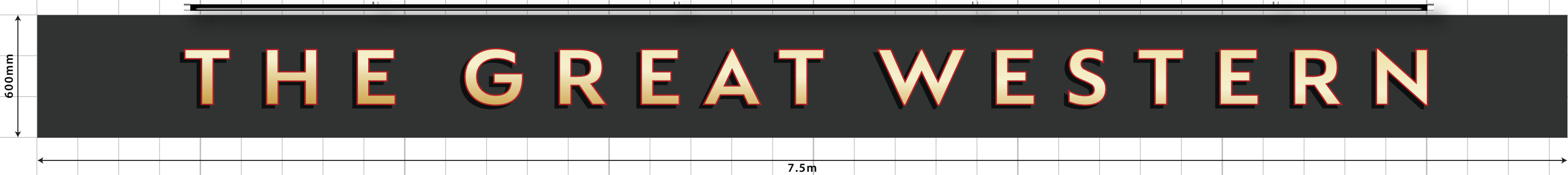
B TWO X GABLE BOARDS WITH APPLIED INDIVIDUAL LETTERS. ONE TO HAVE SIGNWRITTEN SECONDARY TEXT. ILLUMINATED BY TROUGH LIGHTS. SIZE. 2.4m x 1300mm. H.A.G. 3.25m.
