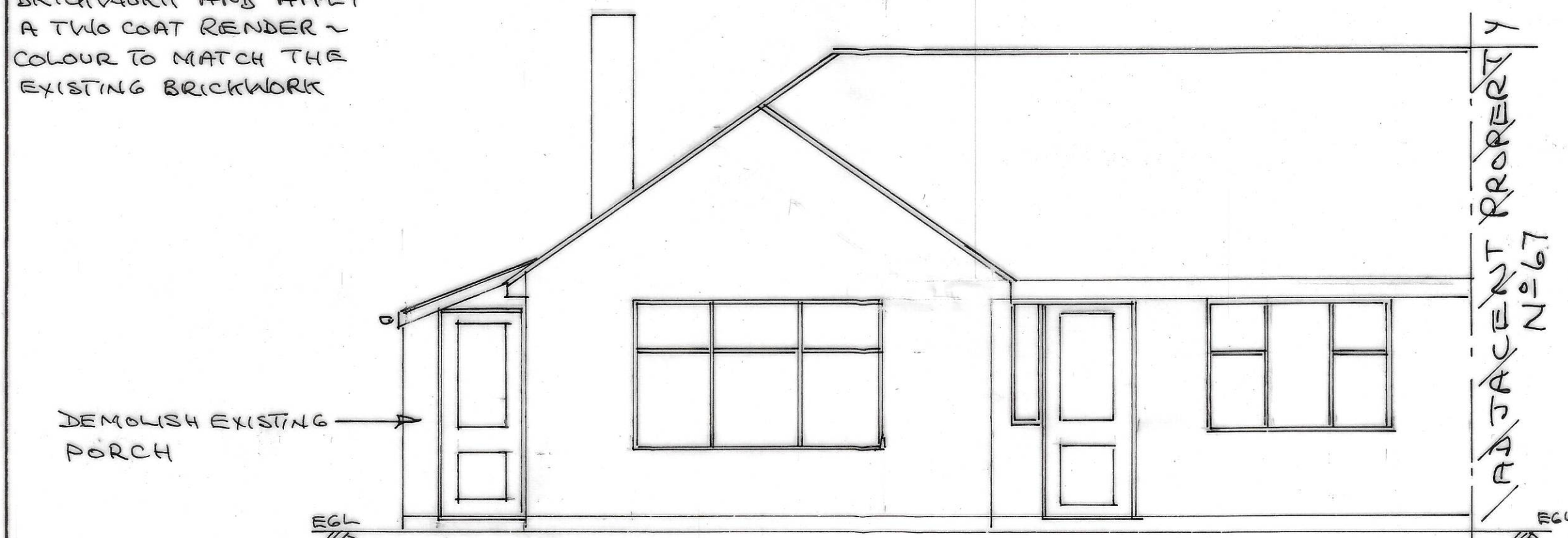
EXISTING SOUTH WEST ELEVATION
