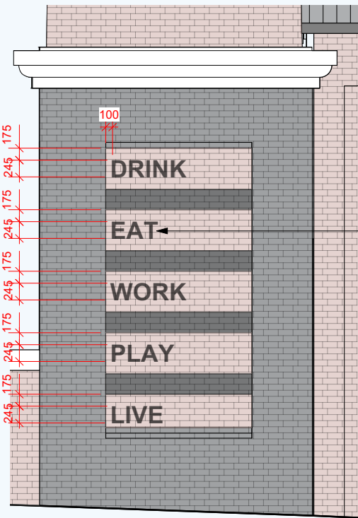
4 Avonside Chimney Base Signage Scale: 1:50
