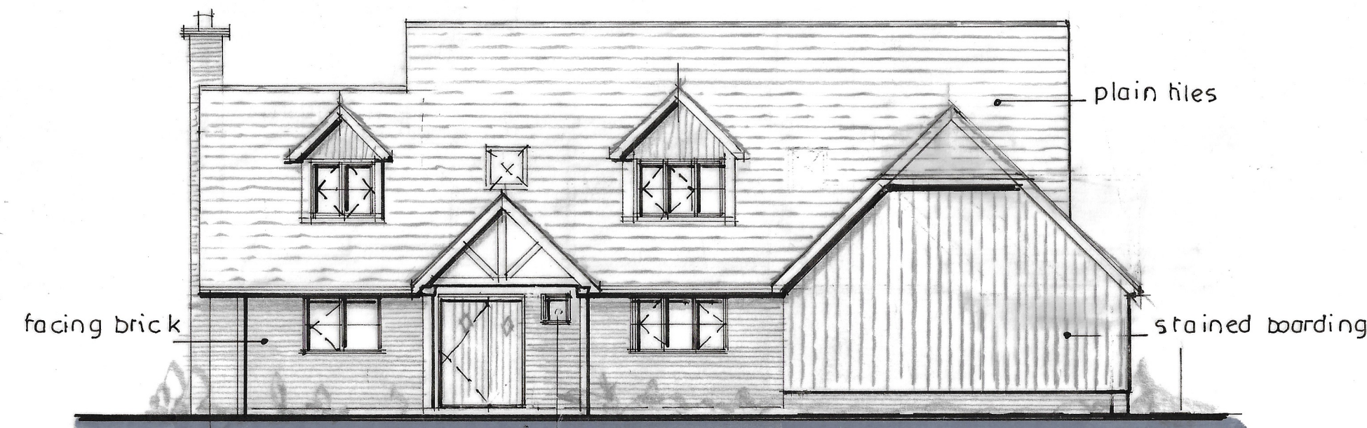
NORTH WEST ELEVATION
