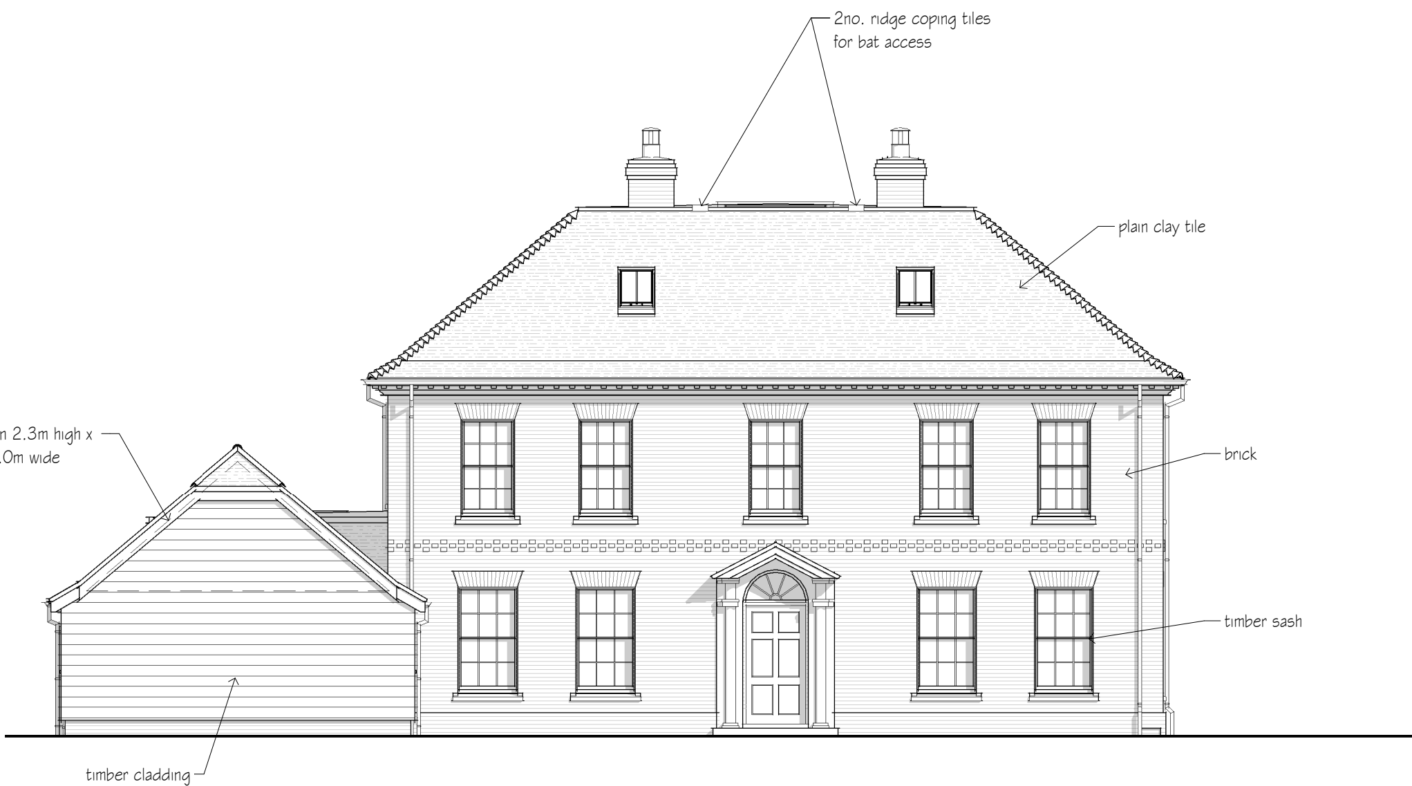
North West Elevation
