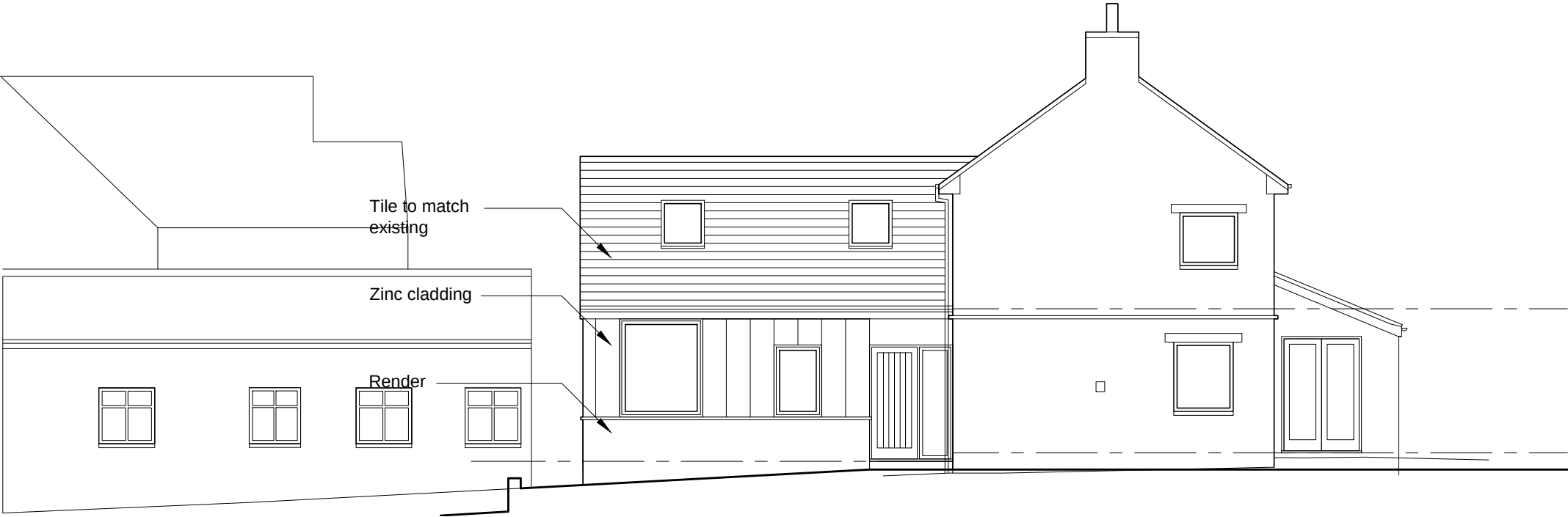
SIDE (SOUTH EAST) ELEVATION
