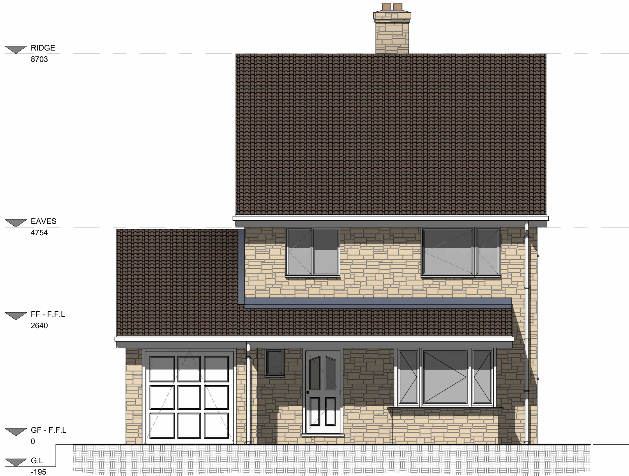
1 EXT_Front Elevation - Materials 1 : 50
