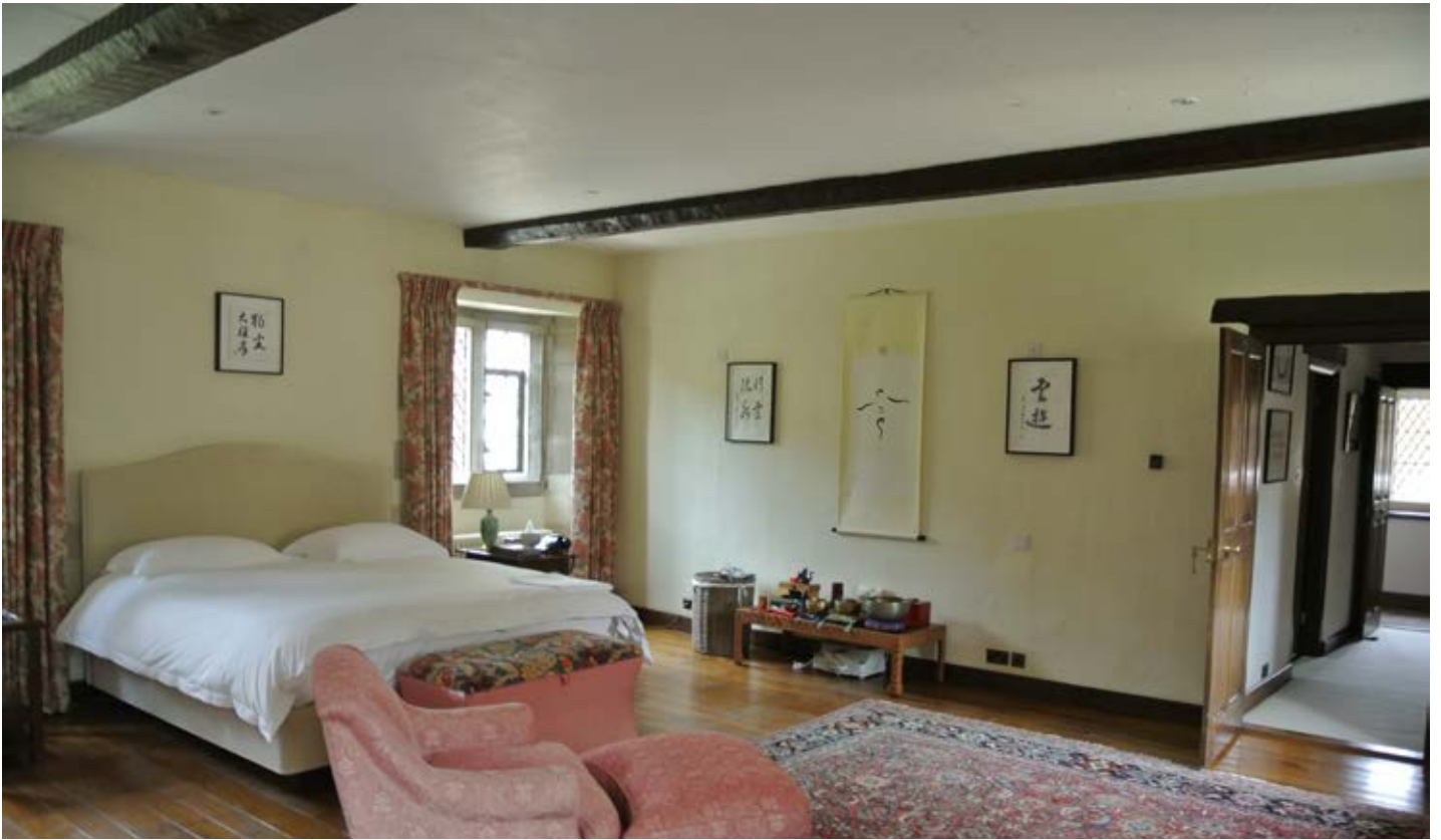
Bedroom with stone mullion casement windows and chamfered beams to ceiling.
