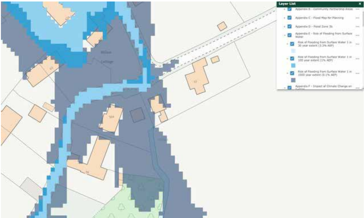
Extract form Wiltshire Council SFRA mapping. Dark Blue area indicates 1in1000 year surface water flooding event to existing driveway area
