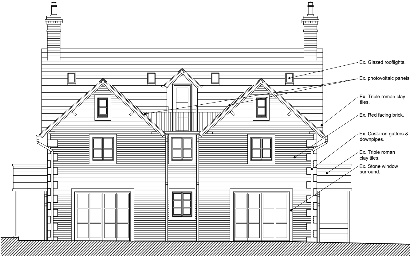
Existing South-West Elevation 1:50 @ A1 (1:100 @ A3)
