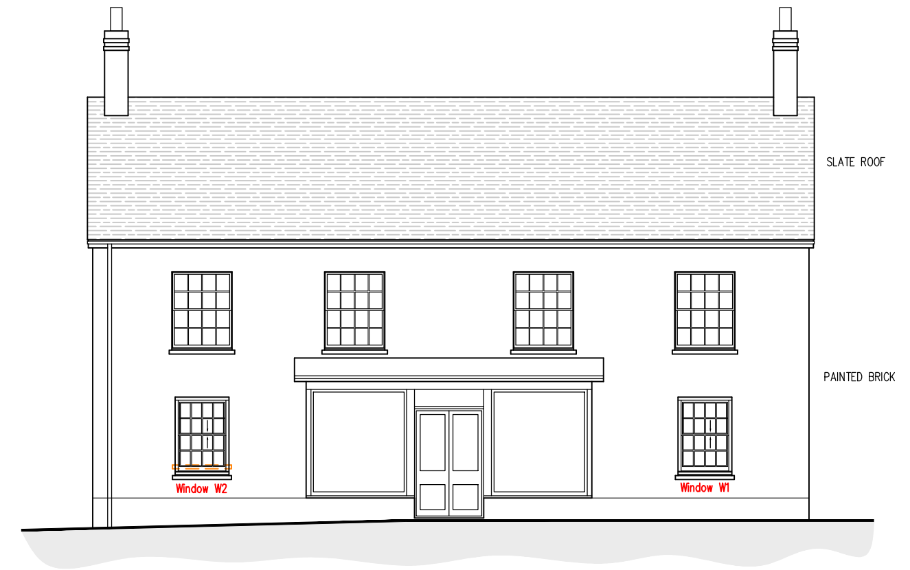
North (Front) Elevation [1:100]
