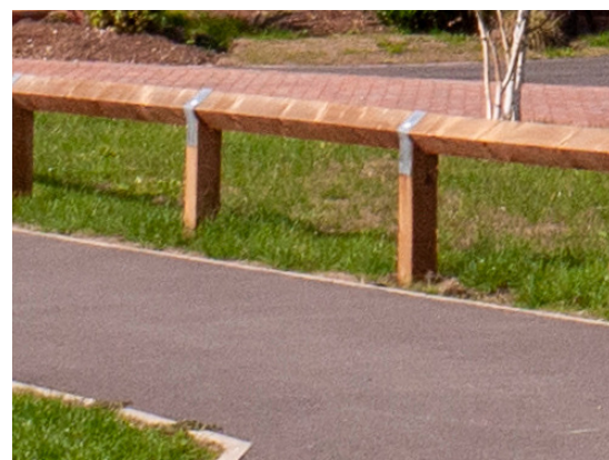
Timber Knee Rail Description: To green spaces, to discourage cut-through routes and protect defensible planting Height: 600mm Colour/Finish: Treated Timber (FSC certified)
