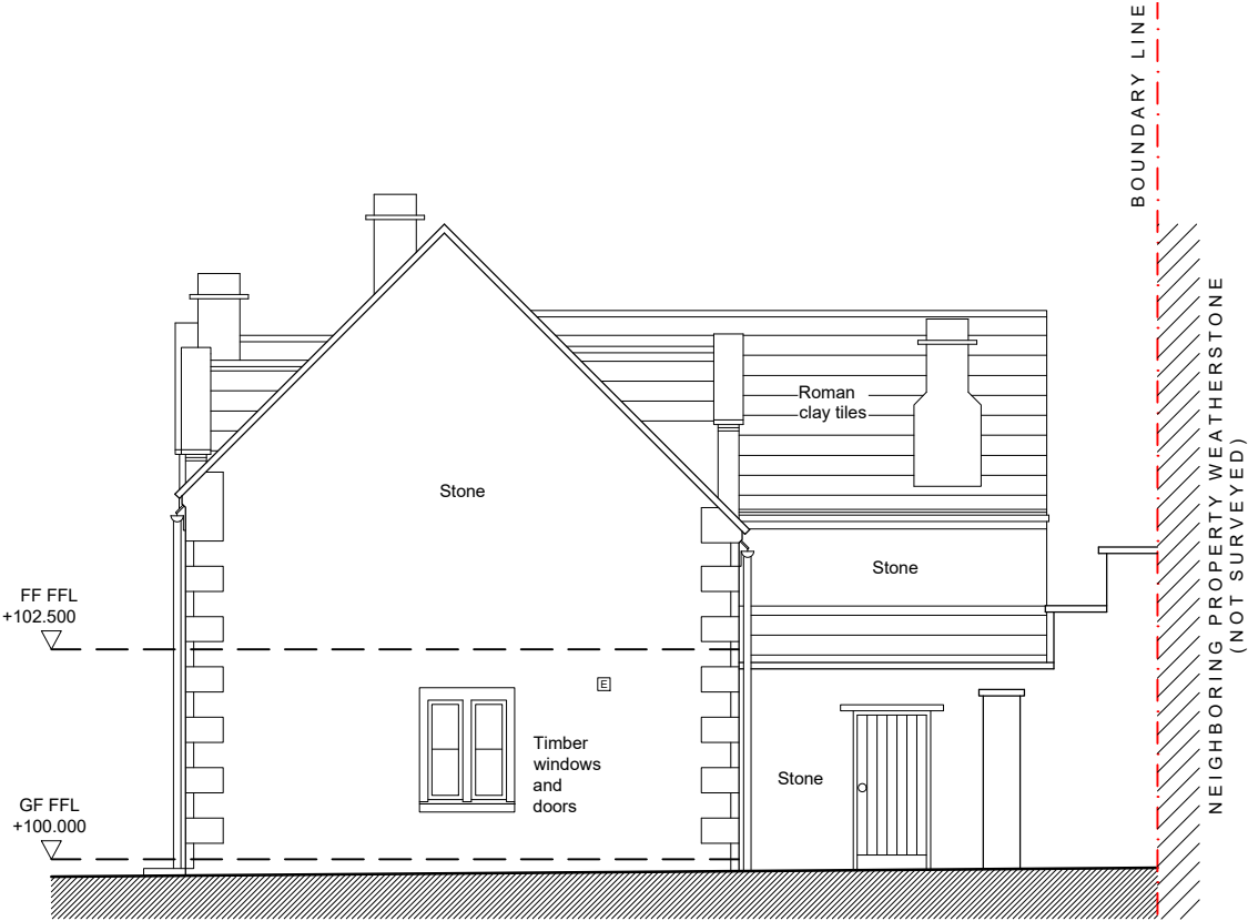
Existing North Elevation
