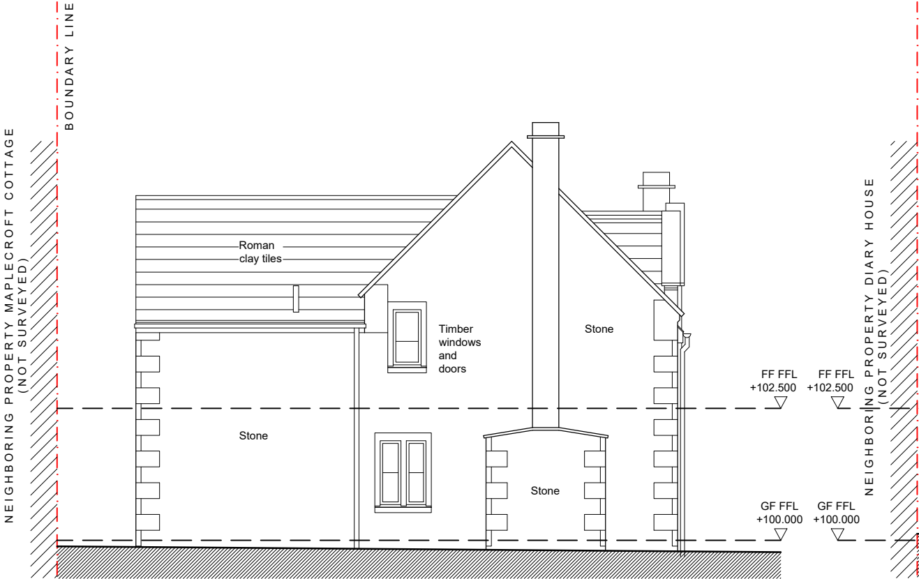
Existing South Elevation
