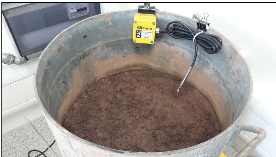
Figure 4 Initial saturation of the bare soil surface.
