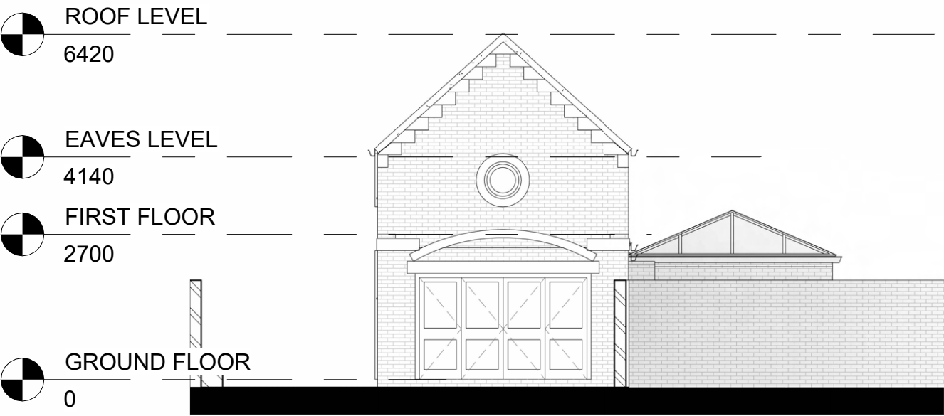
Existing Elevation D
