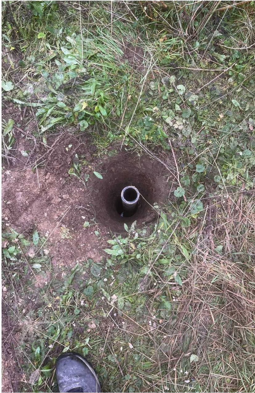
WS2 - with the fitted pipe
