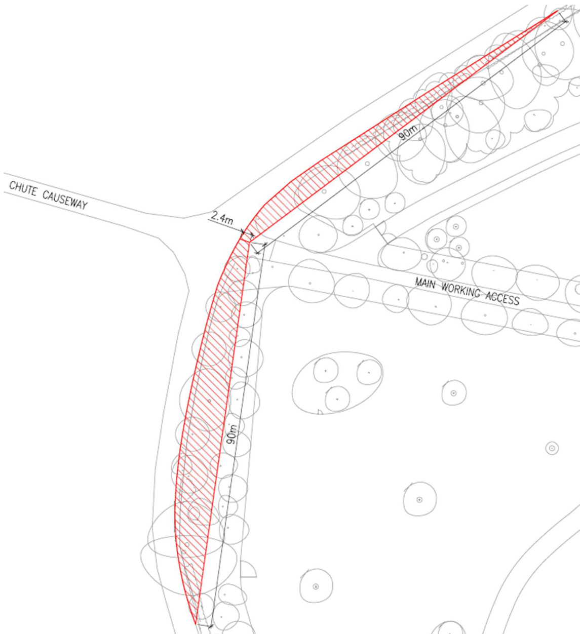
Figure 3-1 Visibility Splay: Main Working Access/Hungerford Lane/Chute Causeway
