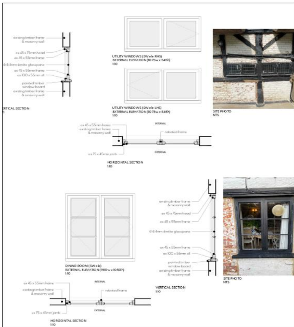
Fig. 29: Design and installation of replacement ground-floor windows (Ben Lilley Design Studio).
