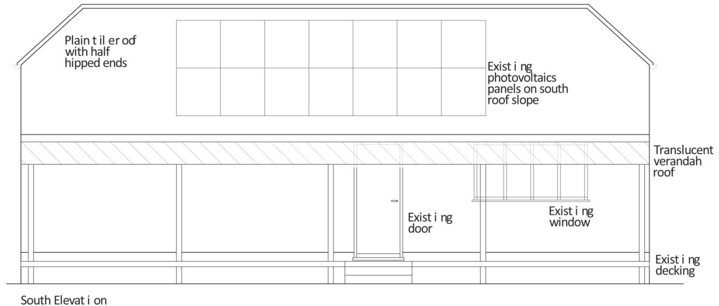
Fig 3.1; Existing South Elevations
