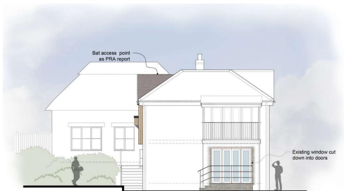
Proposed Southwest Elevation Scale - 1:100
