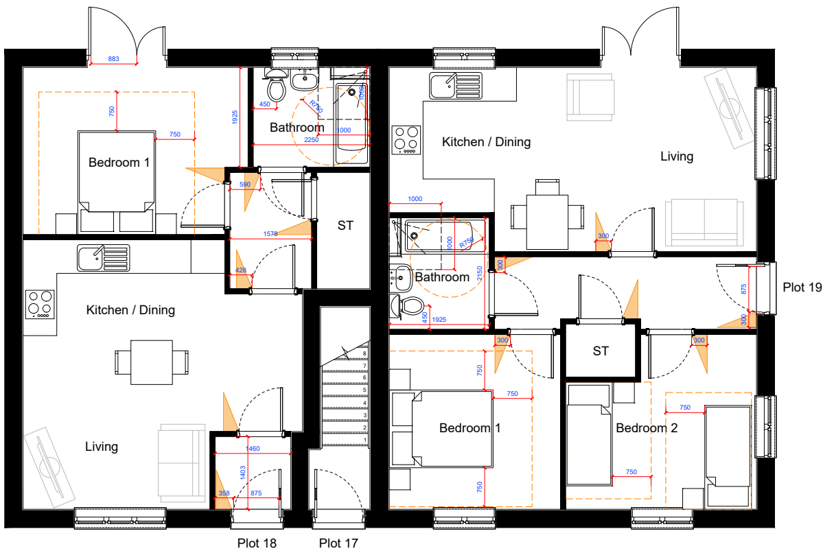
House Type A1M Ground Floor Plan M4(2) - Adaptable
