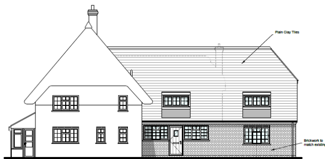
Extension after approval of s73 amendment to a tiled roof.
