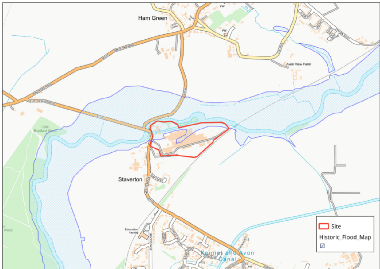
Figure 3.1: Historical Flooding – Environment Agency.
