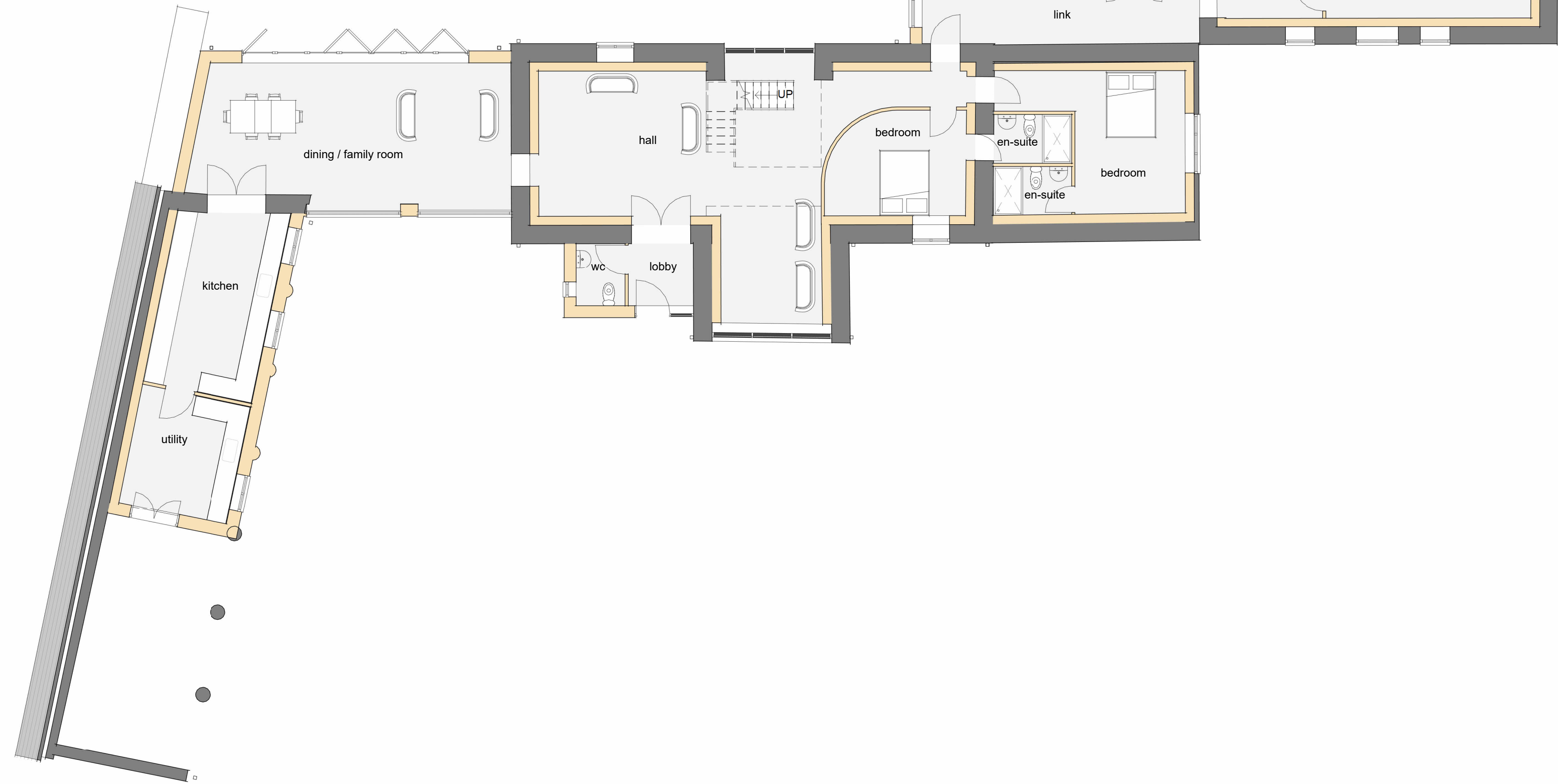
PROPOSED GROUND FLOORPLAN 1 : 100
