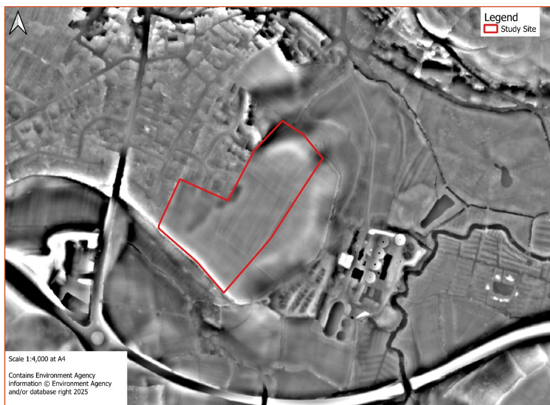
Plate 9 Lidar data of the study site and surrounding area rendered using simplified local relief model analysis
