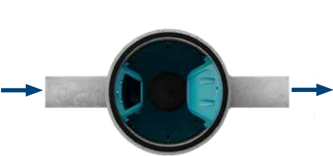
Fig 5. Downstream Defender® Select - online configuration
