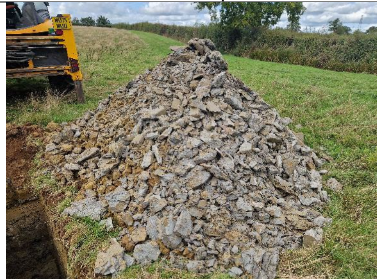
PLATE 40 – Trial Pit Spoil – TP120.
