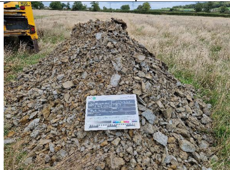
PLATE 56 – Trial Pit Spoil – TP128.
