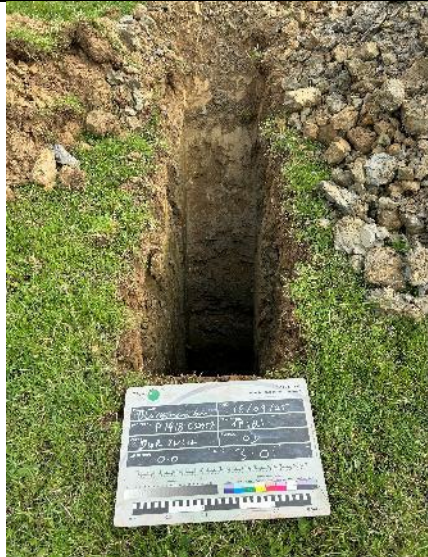
PLATE 41 – Trial Pit Excavation – TP121.
