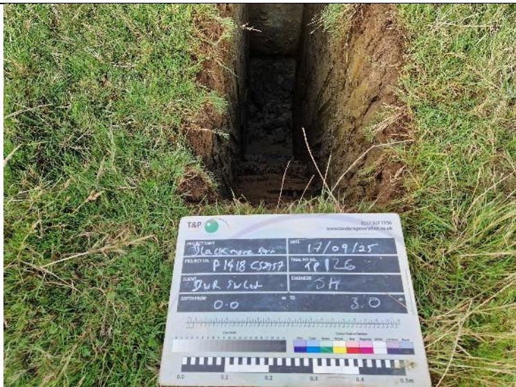
PLATE 51 – Trial Pit Excavation – TP126.
