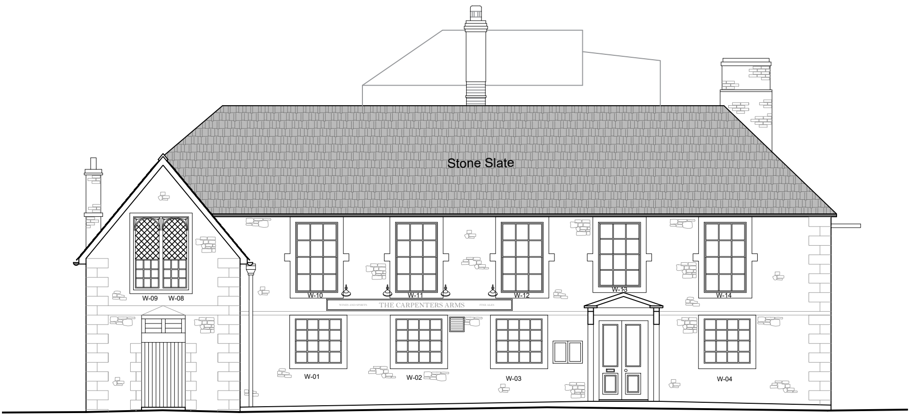
Front (North) Elevation 1:100
