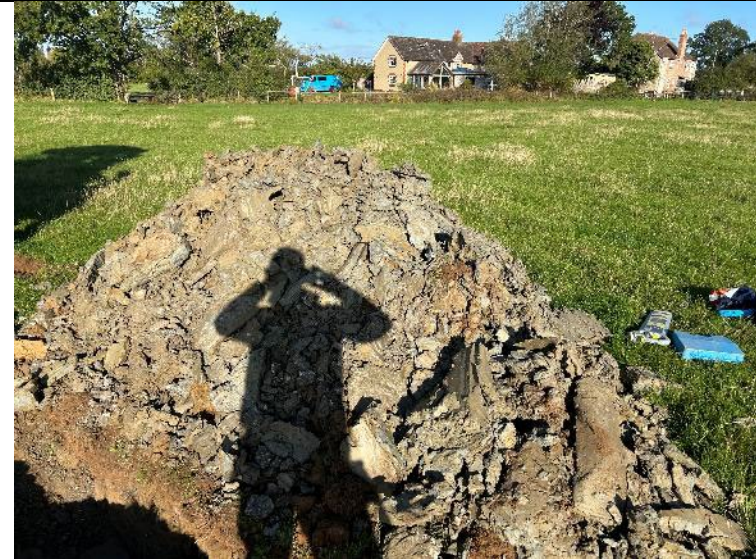
PLATE 02 – Trial Pit Spoil – TP101.
