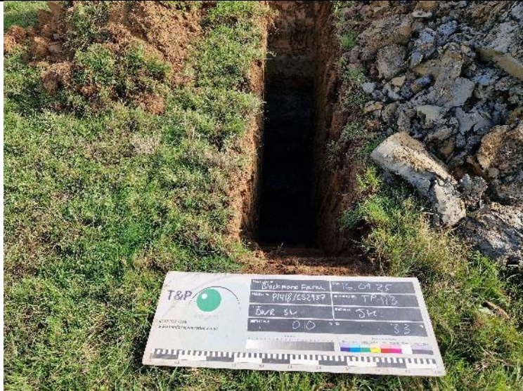
PLATE 25 – Trial Pit Excavation – TP113.
