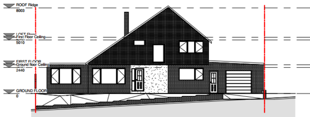
1 EXISTING FRONT ELEVATION 1 : 100
