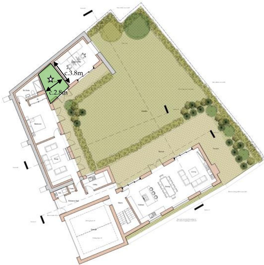
Fig 9: The bat loft will be created above this area of the converted and extended stables with an access for greater horseshoe bats on the northern aspect of the roof.
