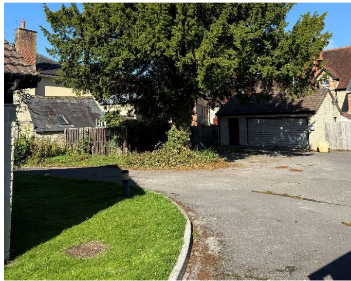
Image 3: T11 with parking area within RPA, garage due for demolition on the right and the soft verge proposed for a NO DIG footpath on the left.
