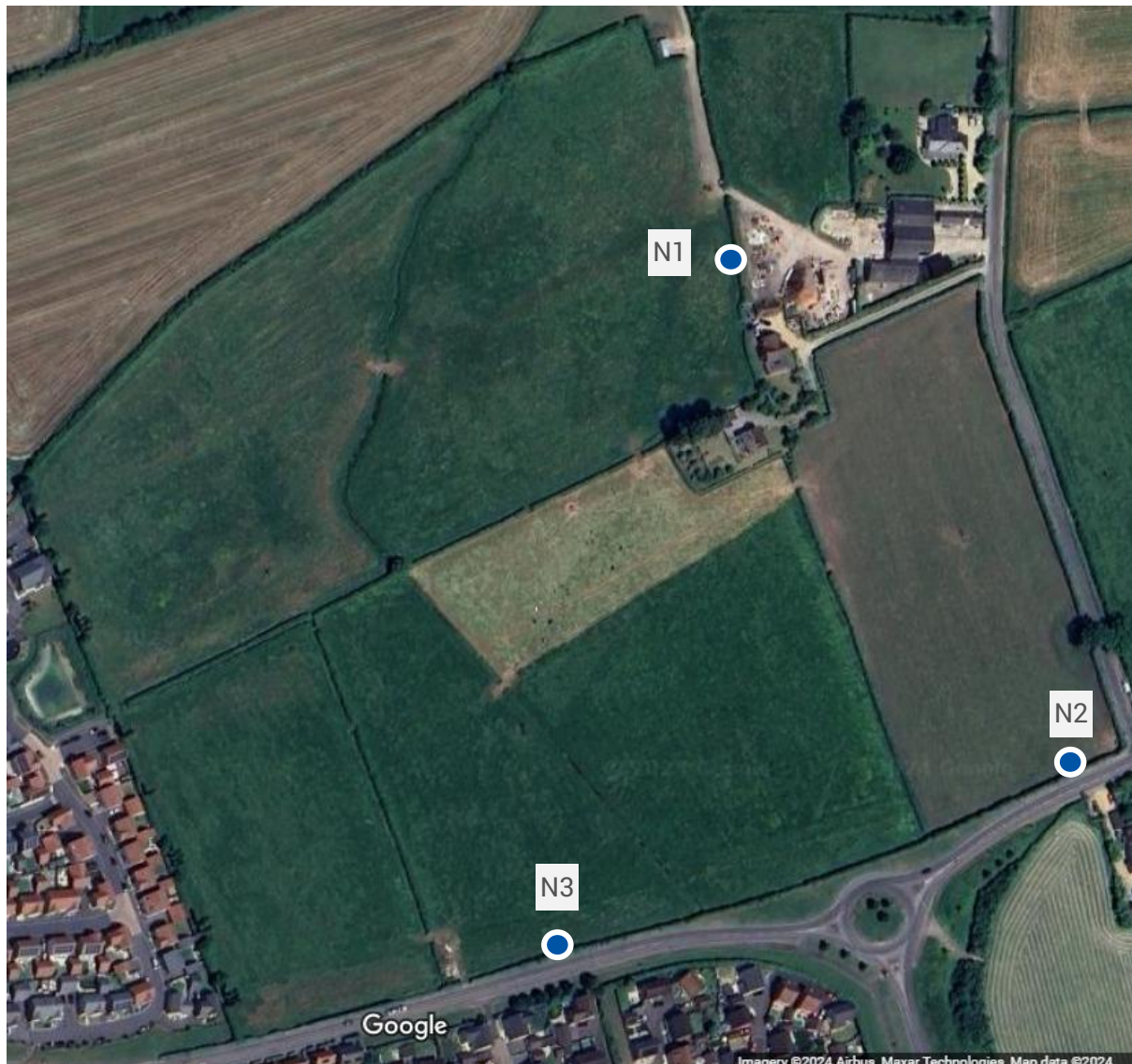
Fig 4.1 Plan showing noise measurement positions N1, N2 and N3
