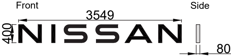
Sign C: Nissan Wordmark Size 2 Individual 3D letters Face Illumination: Internally Illuminated with white LEDs Material: 1mm Hairline S/S Returns 4mm Black/White Acrylic Front Face Scale 1:50 @ A3
