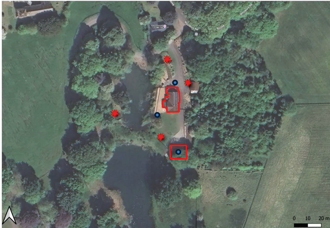
Plate 1: Surveyor and thermal camera locations illustrated by the red stars, with the green circles showing static detector position
