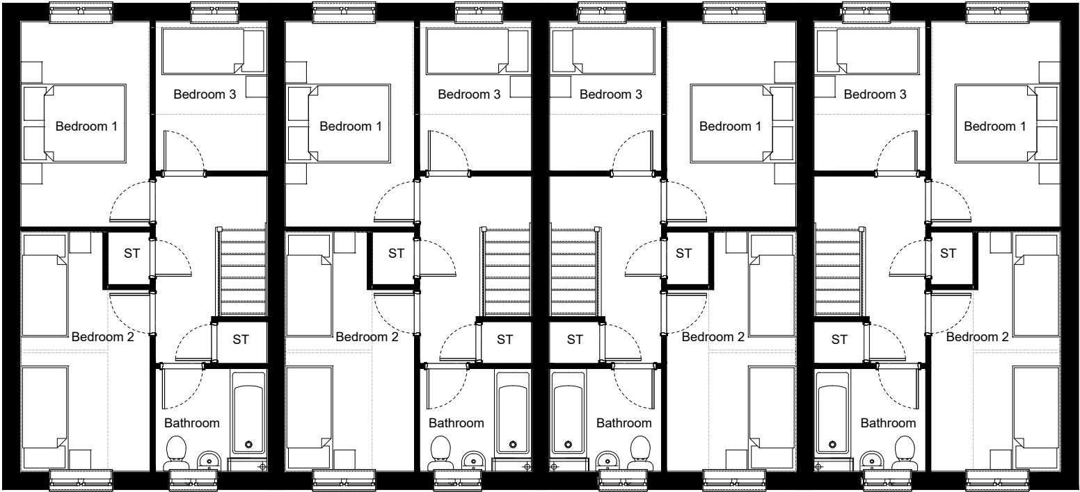
House Type A3 - First Floor Plan
