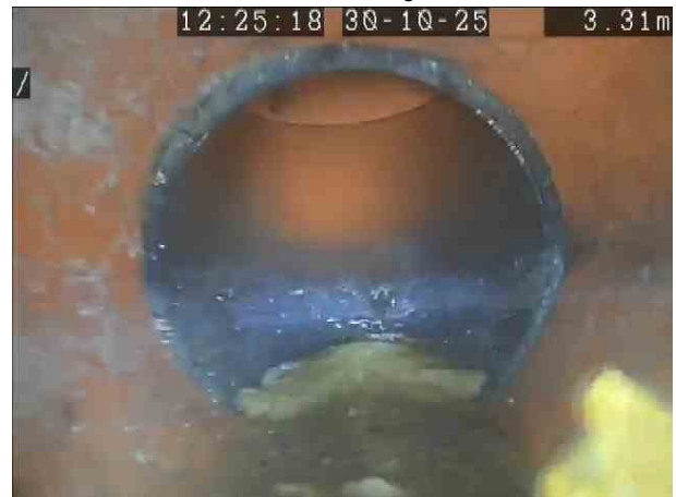
d4a91c55-5049-491c-87b8-bdc95e029d0f.png, 00:00:22, 3.31 m Line deviates up
