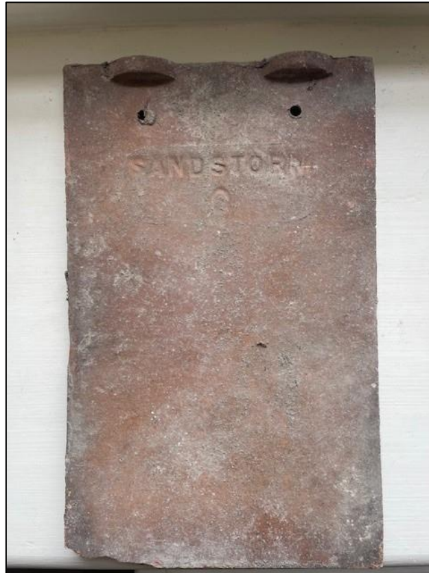
Picture 4: Sandstorm roof tile
