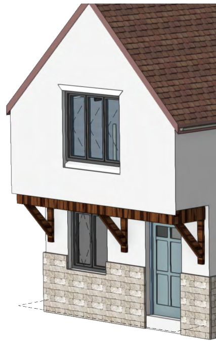
External decorative timber beam and supports over entrance porch to House Type 1
