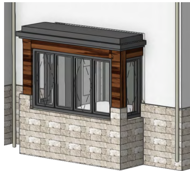
External decorative timber beam and posts to frame bay windows.
