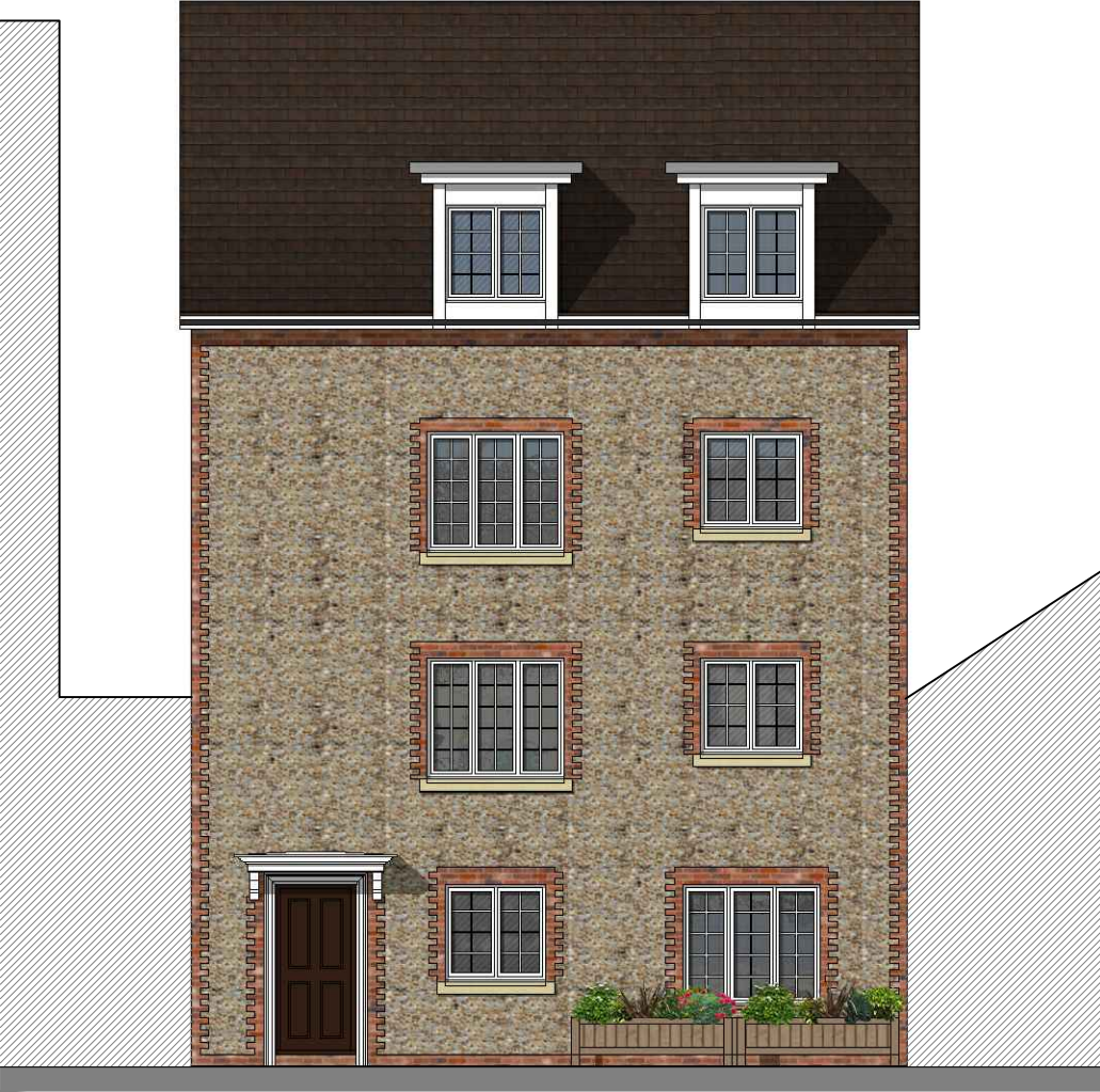
North Elevation Apartment Building (all new construction)
