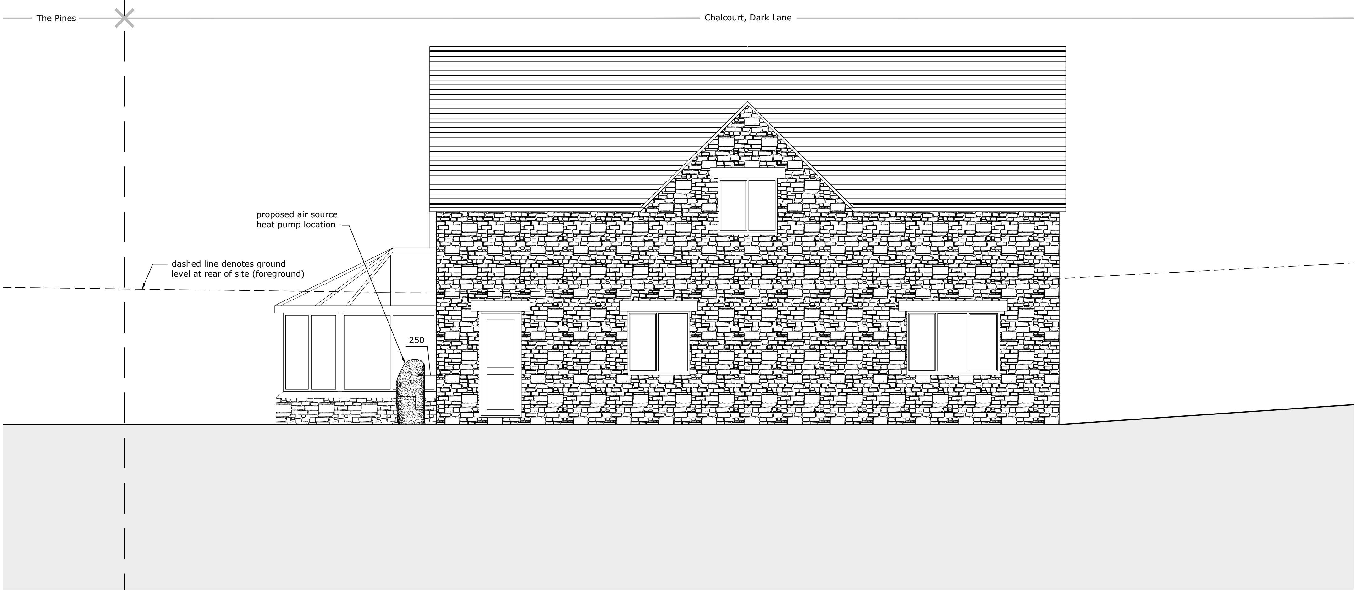
rear elevation (north facing) as proposed 1:50
