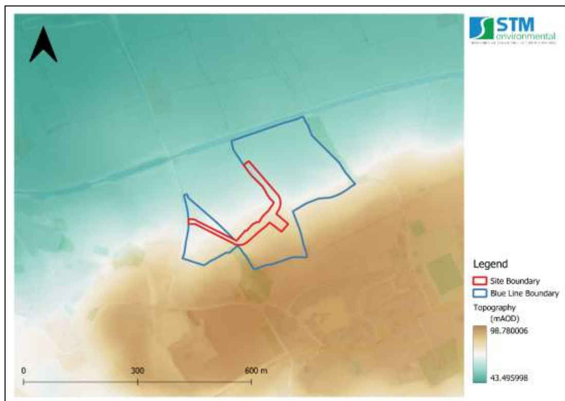
Figure 3 LIDAR DTM Topography within the wider area
