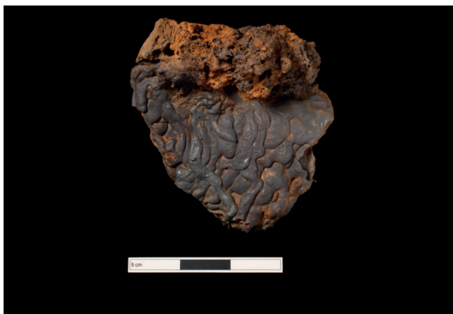
Figure 12. Tap slag with attached furnace lining from deposit 3104 (Trench 31), 0.15 m scale
