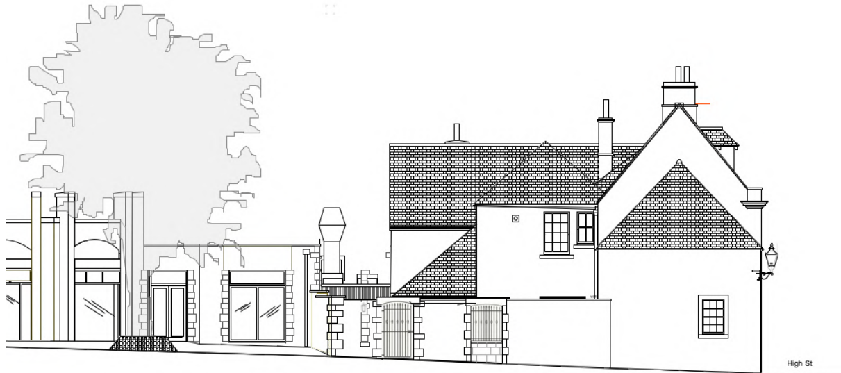
Approved south elevation with flue and jetcowl close to the listed building and visible from the shopping precinct.
