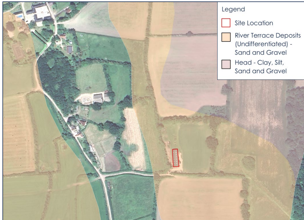
Figure 2-5 BGS Superficial Deposits
