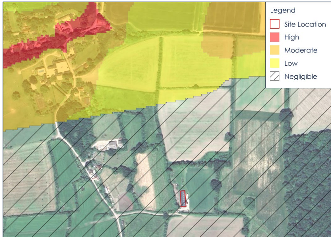
Figure 4-3 GeoSmart Groundwater Flood Risk
